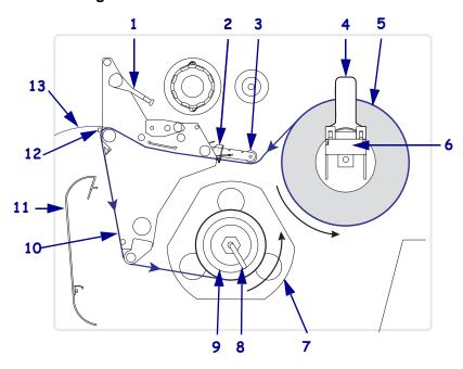
Figure 27 • Media Loaded in Peel-Off Mode
